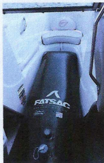
An aftermarket ballast tank designed to hold 370 lbs. of water.
