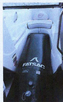
An aftermarket ballast tank designed to hold 370 lbs. of water.
